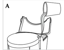
1. Open lid and pour cold water into water reservoir up to the 12-cup level mark on the water window (A). Do not overfill.
