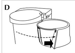
3. Grasp brew basket by small handle and swing open (D). Insert filter into the brew basket, add ground coffee into filter (we recommend one heaping tablespoon for every two cups).
