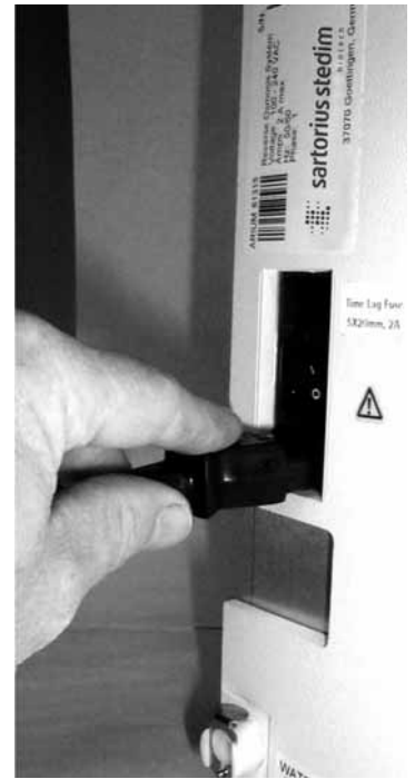
AC power connector port, left-hand side of housing
