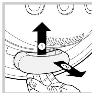
1. Remove the compartment by applying a light pressure to the lower part.
