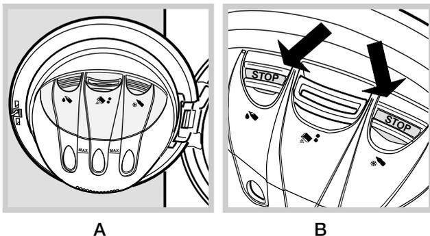
1. Open the porthole door to access the detergent dispenser drawer (see figure A).
