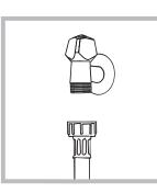
1. Connect the supply pipe by screwing it to a cold water tab using a <sup>3</sup>/<sub>4</sub> gas threaded connection (see figure).
