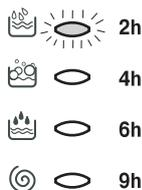
Once the set delay is complete, the flashing LED will turn off and the programme set will start.
