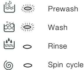
Note: during draining, the LED corresponding to the Spin cycle phase will be turned on.
