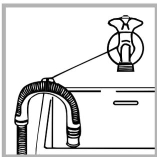
alternatively, place it over the edge of a basin, sink or tub, fastening the duct supplied to the tap (see figure). The free end of the hose should not be underwater.
