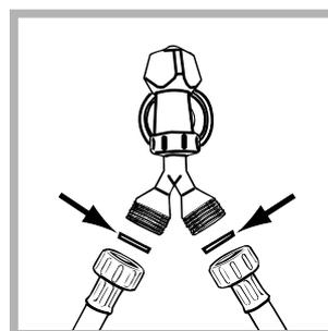
1. Connect the supply pipe to the water mains using a gas 3/4 attachment, fitting the rubber gasket and the filter supplied with the appliance and ensuring that they are firmly tightened to the taps.
