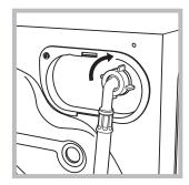
2. Connect the other end of the water inlet hose to the washing machine, screwing it onto the applian-
