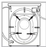
3. Remove the **4** protective screws and the rubber bush with the respective spacer, situated on the rear of the appliance (see also the installation leaflet).
