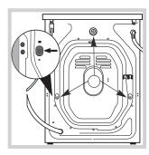
3. Remove the **3** protective screws and the rubber bush with the respective spacer, situated on the rear of the appliance (see also the installation leaflet).
