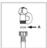
screw the latter onto a cold water tap with a 3/4 gas threaded mouth (see figure). Before making the connection, allow the water to run freely until it is perfectly clear.
