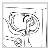
screwing it onto the appliance's cold water inlet, situated on the top right-hand side on the rear of the appliance (see figure).
