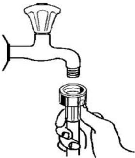
Connect the cold water supply hose to a threaded 3/4 (inch) connector and make sure that it is fastened tightly in place. If the water pipes are new or have not been used for an extended period of time, let the water run to make sure that the water is clear and free of impurities. If this precaution is not taken, there is a risk that the water inlet can get blocked and damage the appliance.
