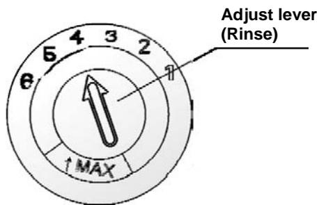
The rinse aid dispenser has six or four settings. Always start with the dispenser set on "4". If spots and poor drying are problems, increase the amount of rinse aid dispensed by removing the dispenser lid and rotating the dial to "5". If the dishes still are not drying properly or are spotted, adjust the dial to the next higher number until your dishes are spot-free. The recommended setting is "4". (Factory value is "4".)
