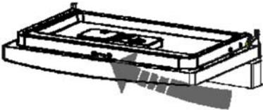
To clean the edge around the door, you should use only a soft warm, damp cloth. To avoid penetration of water into the door lock and electrical components, do not use a spray cleaner of any kind.
