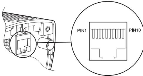
Figure 4. RJ45-10 Connector
