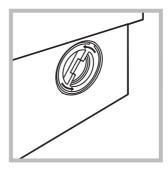
2. unscrew the lid rotating it anti-clockwise (see figure): a little water may trickle out. This is perfectly normal;
