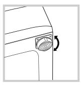
2. If the floor is not perfectly level, compensate for any unevenness by tightening or loosening the adjustable feet (see figure), the angle of inclination, measured according to the worktop, must not exceed 2°.
