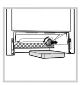
2. unscrew the lid rotating it in anti-clockwise. A little water may trickle out (about 1 liter). Put a little container under the hole
