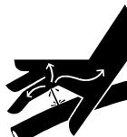
Hydraulic fluid under pressure. Do NOT use any part of your body to locate a hydraulic leak. Escaping fluid under pressure can cause severe injury or death. If injury results from escaping hydraulic fluid, seek immediate medical attention to avoid serious bodily injury.
