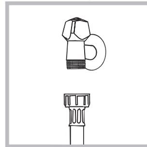
1. Connect the supply pipe by screwing it to a cold water tap using a 3/4 gas threaded connection (see figure).
