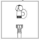
1. Connect the supply pipe by screwing it to a cold water tap using a 3/4 gas threaded connection (see figure).
