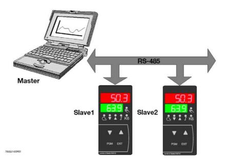
A master computer controls the exchange of data and can address up to 99 controllers via device addresses (slaves).
