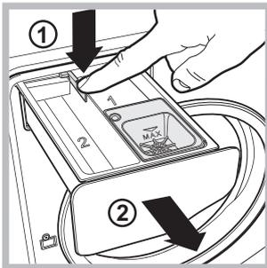
To remove the drawer, press lever (1) and pull the drawer outwards (2) (see figure). Wash it under running water; this procedure should be repeated frequently.
