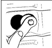
Unscrew the bolt using a 13mm spanner.
