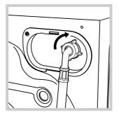
1. Connect the inlet hose to the machine, by screwing it into the cold water inlet on the upper right hand side of the back of the machine (see figure).
