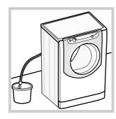
1. Remove the plug from the electricity socket; 2. Make sure that the water level inside the machine is lower than the door opening; if this is not the case remove excess water using the water outlet hose, collecting it in a bucket as shown in the *figure*;
