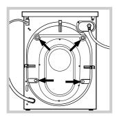
2. Remove the four transit bolts and the rubber bush with the respective spacer, situated on the rear of the appliance.
