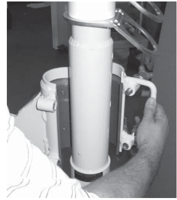
Figure 11 - Anchor Post Set Up
