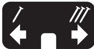
TO SELECT ACTUATION MODE SLIDE SWITCH LEFT OR RIGHT.
