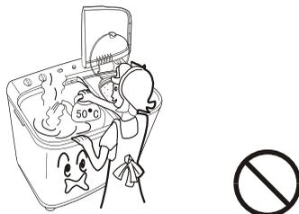
In case the washing machine is installed on ground with carpet, do not block the ventilation hole with carpet.
