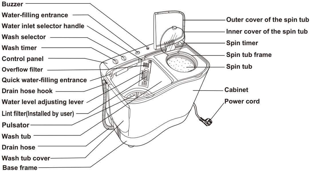
Note: Different machine, the form of control panel is different.
