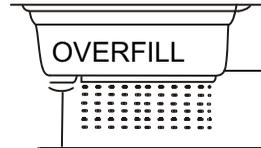
If you find water flowing out here, please twist the water tap to limit the water filling.
