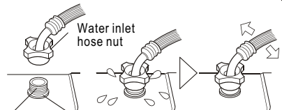
Water inlet valve jointer Water absorption cushion.
