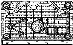
Ventilation hole at the bottom of the washing machine
