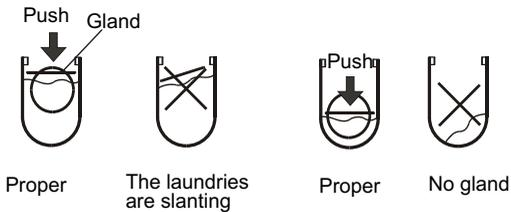
(2) Close the inner and outer cover of the spin tub.
