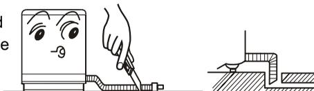
4. If extra drain hose is needed, please make separate purchase. The inner diameter of the extra hose shall not less than 40mm, and the length shall not exceed 1.5m.
