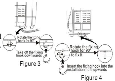
Install the two drain hose fixing hooks taken out into the installation hole at the other side of the base frame (to aim at the installation hole accurately you can lean the washing machine forward slightly). Then rotate for 90° (As per Figure 4).
