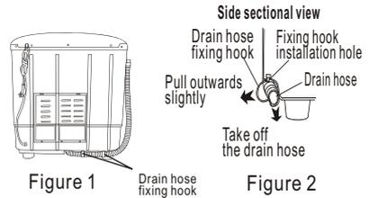
Rotate the drain hose fixing hook for 90° to take it out from the installation hole (As per Figure 3).
