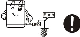
When the machine is normally using, please put the power plug at the location easily to be inserted and extracted by hand. Be sure to pull the plug off when there's power failure, or the machine is being moved, cleaned or when it is idle.
