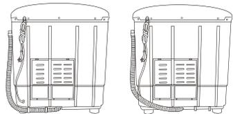
Then hang the drain hose into the hanging hole at the spin tub side. (As per Figure 5).
