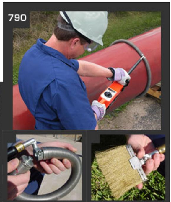
**PosiTector UTG (Ultrasonic Thickness Gage)**
