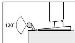
When the TV is placed on a cabinet or table: Place the 3D Sync Transmitter in the middle of the TV along the front edge of the Table-top stand or TV stand.
