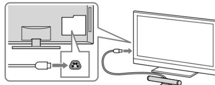
Turn on the TV and confirm that the 3D menu items appear on the OPTIONS menu list. Be sure to turn off the TV once in order for the TV to recognize the 3D Sync Transmitter. Refer to TV's instruction manual for details on how to enjoy 3D viewing.
