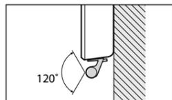
If the TV is mounted on a wall, attach the 3D Sync Transmitter to the TV (top center or bottom right-of-center), using double-sided tape.
