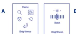
Press the side keys ⚡ on the multi-function button (9) to move the cursor to the backlit LCD display brightness adjustment, 'Brightness' icon, ☀️ (A). When the cursor is on the relative icon, press the centre key on the multi-function button (9) to confirm access to the backlit LCD display brightness adjustment sub-menu (B).
