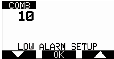
Figure 3-6. Sensor Alarm Setup
