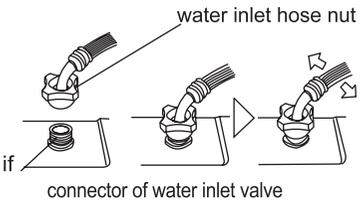
2. slightly shake the water inlet hose nut to see if it is tightly and properly fixed.
