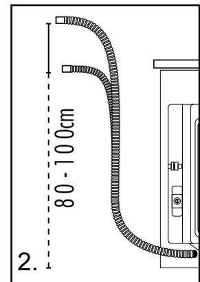
**Note: The drain hose should not be submerged in water and should be securely fixed and leak-free. If the drain hose is placed on the ground or if the pipe is at a height of less than 80cm, the washing machine will continuously drain while being filled (self-siphoning).**
