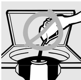
*Do not pour anything into the agitator if the agitator cap or dispenser is removed.*
