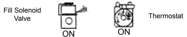
3) "HI" electrode circuit closes. Dual Level Control turns power off to fill valve and continues power to thermostat.
