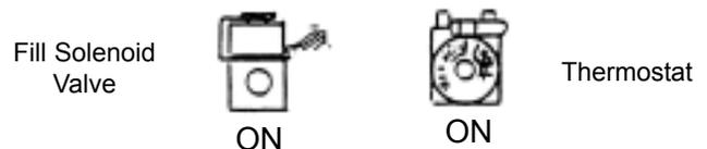
5) "XL" electrode circuit now opens. Power to thermostat is turned off. Power to fill valve remains on.
