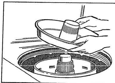
5. After loading clothes in the Mini-Basket tub, be sure to replace the Filter-Flo pan. The pan serves as a lid to keep the clothes in the Mini-Basket tub.
