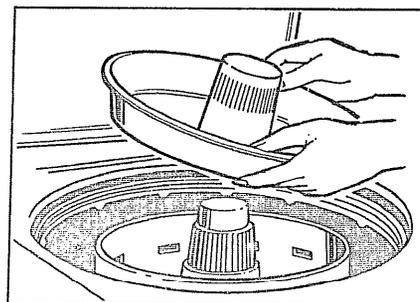
5. Replace the Filter-Flo pan. The pan serves as a lid to keep the clothes in the Mini-Basket tub.
