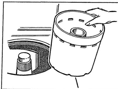
2. Place Mini-Basket tub on agitator. Pull the agitator toward the front of the machine for easier installation and removal of Mini-Basket tub.
