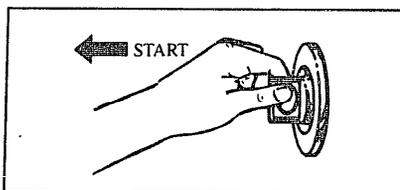
3. Pull Cycle Selector knob to start washer. Cycle will be completed automatically.
