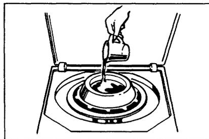
7. Add fabric softener, if desired. Place the Fabric Softener Dispenser on the Filter-Flo pan. Pour 1 teaspoon (5 ml) of concentrated softener or 1 tablespoon (15 ml) of diluted softener into a standard measuring cup. Add enough water to fill the cup ½ full. Pour the diluted softener into the dispenser. See page 9 for dispenser instructions.
