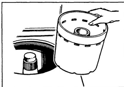
2. Place Mini-Basket tub on agitator. Pull the agitator toward the front of the machine for easier installation and removal of Mini-Basket tub.
