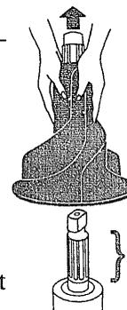
When replacing the agitator, carefully lower straight down onto the shaft so that it fits into the slots. Then apply downward pressure until agitator snaps into its normal position.
