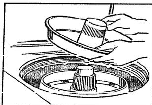
6. Add bleach, if desired. Measure carefully and pour recommended amount of liquid bleach—1/4 cup (60 ml)—directly into the bleach dispenser. See How to Use the Bleach Dispenser section for dispenser usage instructions.
