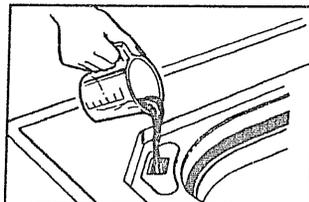
7. Add fabric softener, if desired. Place the fabric softener dispenser on the Filter-Flo pan. Pour 1 teaspoon (5 ml) of concentrated softener or 1 tablespoon (15 ml) of diluted softener into a standard measuring cup. Add enough water to fill the cup 1/2 full. Pour the diluted softener into the dispenser. See How to Use the Fabric Softener Dispenser for dispenser usage instructions.
