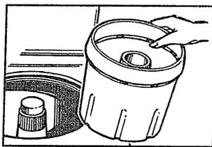
3. Put 1/4 to 1/3 cup (60 to 80 ml) detergent in the bottom of the Mini-Basket tub.
