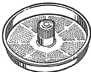
• LID FOR THE MINI-BASKET—After loading clothes in the Mini-Basket tub, be sure to replace the Filter-Flo pan. The pan serves as a lid to keep the clothes in the Mini-Basket tub.
