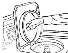
Do not use Mini-Basket tub when washing regular loads. You'll find complete details on how and when to use the Mini-Basket tub in How to Use the Mini Basket™ Tub section.
