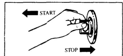
**4** Pull Cycle Selector Knob out to start the washer. If you wish to change setting after washer has started, push Cycle Selector Knob in to stop the washer and reset to the new position. Setting can be changed at any time.
