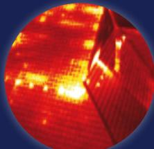
Picture taken of a roof with grow lights. Underneath, due to moist the heat is even better to see, moist is one of the best conductors for heat. (Mostly uses for an insulator)
