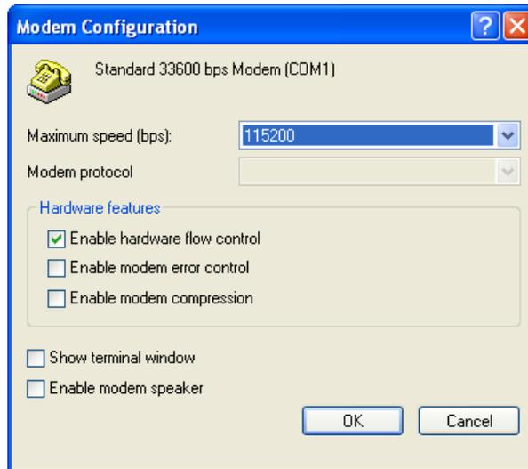
Figure 3-24: Modem Configuration
