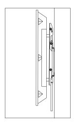
If you think the ribbon(5) is too long, You can hide it at the back of the televesion, once you want to uninstall the TV, it can help you to take out the brackets. When the screws become loose, you can use a wrench to tighten it.
