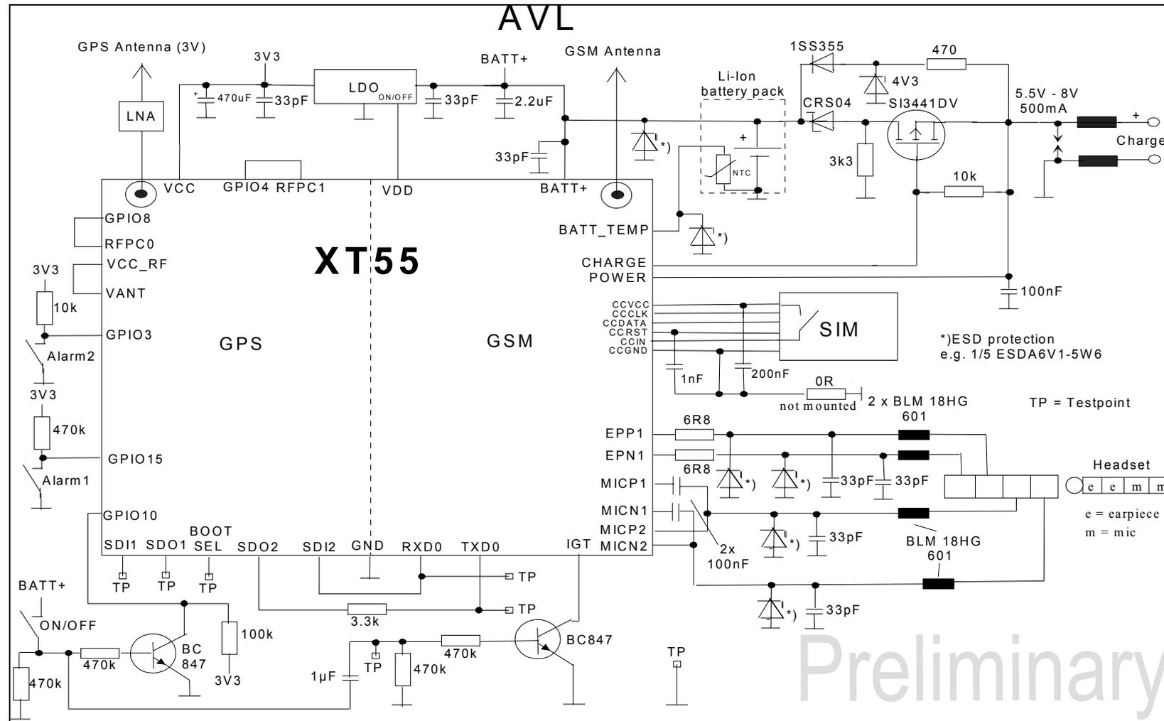
Figure 13: Example application of XT55 module with integrated AVL software
