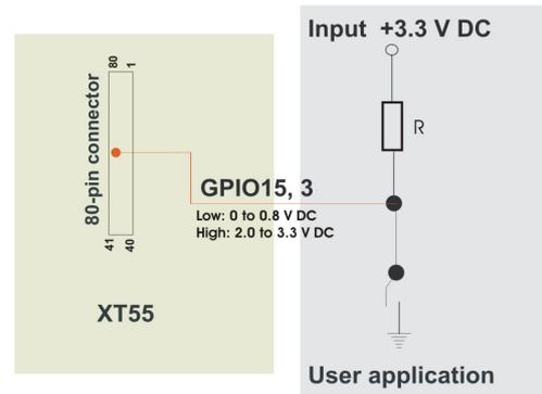
Figure 12: Connection example for GPIO 15 and GPIO 3
