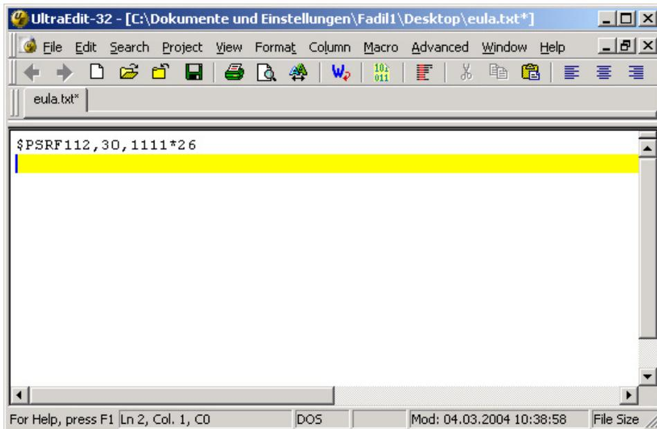
Figure 8: Example of an extended NMEA command
