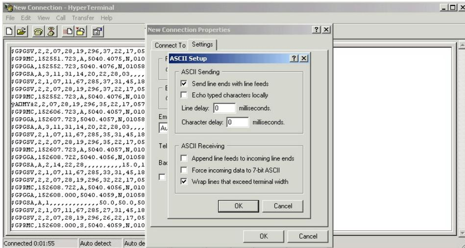
Figure 7: ASCII setup
