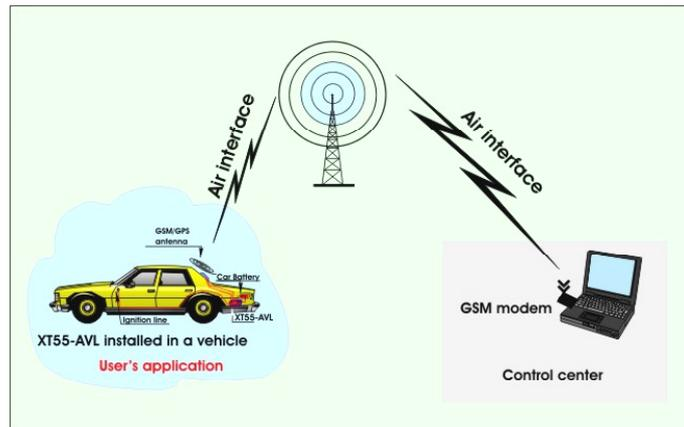
Figure 1: Simplified presentation of the AVL client-server architecture.
