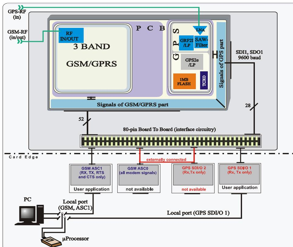
Figure 2: Block diagram of XT55 with AVL application
