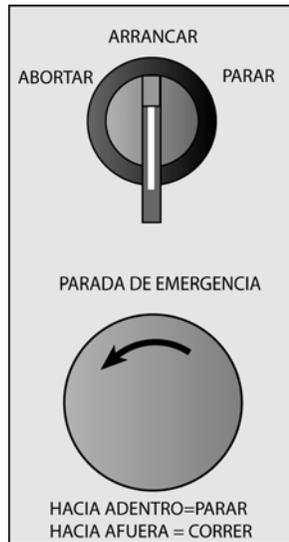
Figure 8-2. Interruptor de Batching
