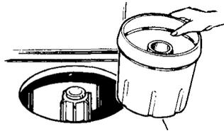
3. Put detergent in the bottom of the Mini-Basket tub before loading clothes (about the same amount you would use for a small load in the regular wash basket). See How Much Detergent Should You Use section.
