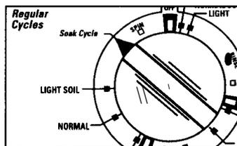
Start the washer. After washer fills and begins to agitate, push in the Cycle Selector knob and turn to **SOAK CYCLE**. Pull out the Cycle Selector knob to complete the cycle.
