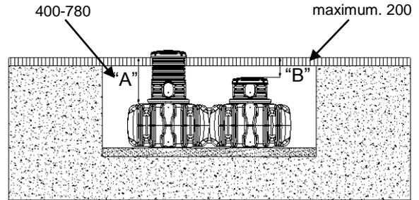
The tanks may not be installed in areas used by passenger cars.
