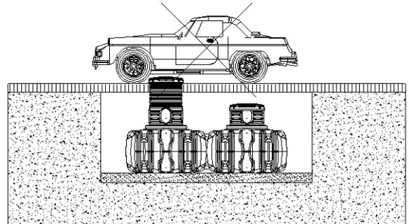
The tanks may not be installed in the groundwater/artesian water. Even if it is expected that groundwater/artesian water occurs only occasionally, this must be led off by a drainage facility.
