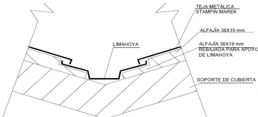
THE TILES MAY BE BUTTED TOGETHER TO FORM A CLOSED VALLEY OR 50mm WIDE MINIMUM OPEN VALLEY MAY BE FORMED. CUT EDGES OF TILES MUST BE BENT DOWN TO FORM DRIP.
