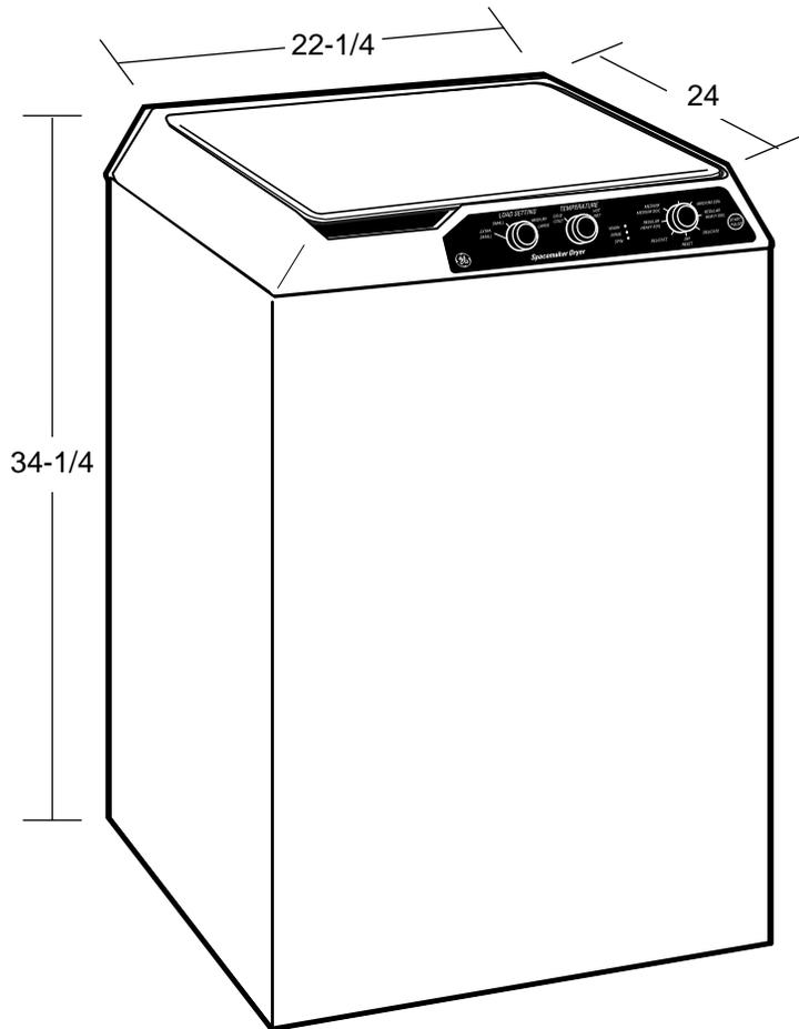
**Washer Note:** Washer wall outlet must be located within 36" of service cord entry. Wall outlet must not be located behind dryer.
