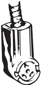
Typical 30 amp receptacle for use where local codes permit use of flexible type power supply cord (pigtail).
