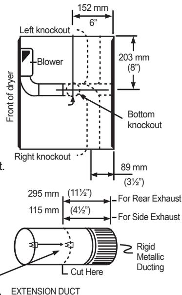
It is important to replace the ground clip after cutting the exhaust duct, (on rear exhaust model).
