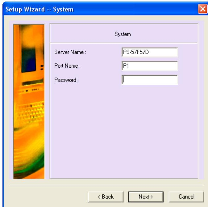
You can give the Print Server a name in your network. Enter this at "Server Name". The "Port Name" represents the name of the port where your printer is connected to.
