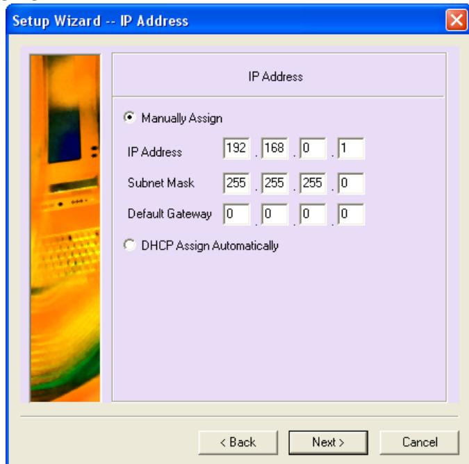
When needed, you can change the IP address and Subnet Mask of your Print Server. You can also set the configuration to "DHCP Assign Automatically" if you have a DHCP server in your network.
